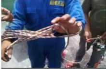
and kept in its usual place for standby for use in a drill or in an emergency. The rope packed in the figure of '8' manner when released
